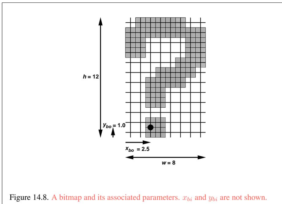
Figure 14.8. A bitmap and its associated parameters.  $x_{bi}$  and  $y_{bi}$  are not shown.
