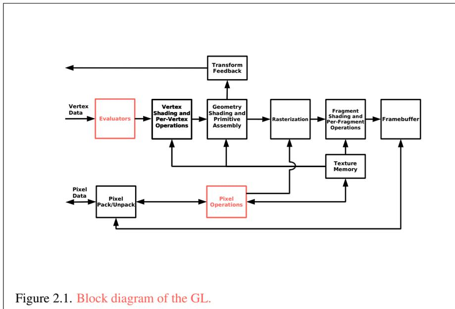
Figure 2.1. Block diagram of the GL.
