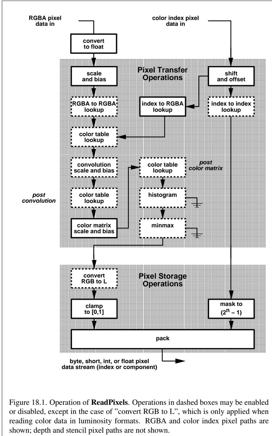
Figure 18.1. Operation of **ReadPixels**. Operations in dashed boxes may be enabled or disabled, except in the case of "convert RGB to L", which is only applied when reading color data in luminosity formats. RGBA and color index pixel paths are shown; depth and stencil pixel paths are not shown.
