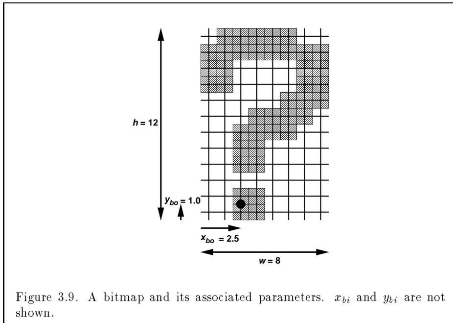
$w$  and  $h$  comprise the integer width and height of the rectangular bitmap, respectively.  $(x_{bo}, y_{bo})$  gives the floating-point  $x$  and  $y$  values of the bitmap's origin.  $(x_{bi}, y_{bi})$  gives the floating-point  $x$  and  $y$  increments that are added to the raster position after the bitmap is rasterized. *data* is a pointer to a bitmap.
