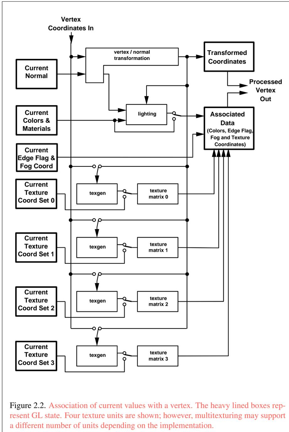
Figure 2.2. Association of current values with a vertex. The heavy lined boxes represent GL state. Four texture units are shown; however, multitexturing may support a different number of units depending on the implementation.
