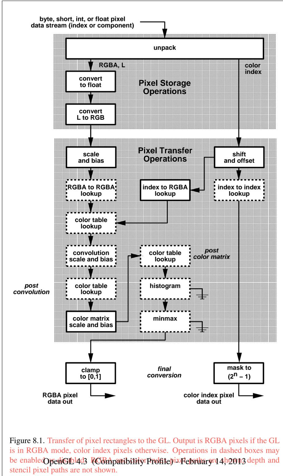
Figure 8.1. Transfer of pixel rectangles to the GL. Output is RGBA pixels if the GL is in RGBA mode, color index pixels otherwise. Operations in dashed boxes may be enabled or disabled. OpenGL 4.3 (Compatibility Profile) - February 14, 2013. depth and stencil pixel paths are not shown.
