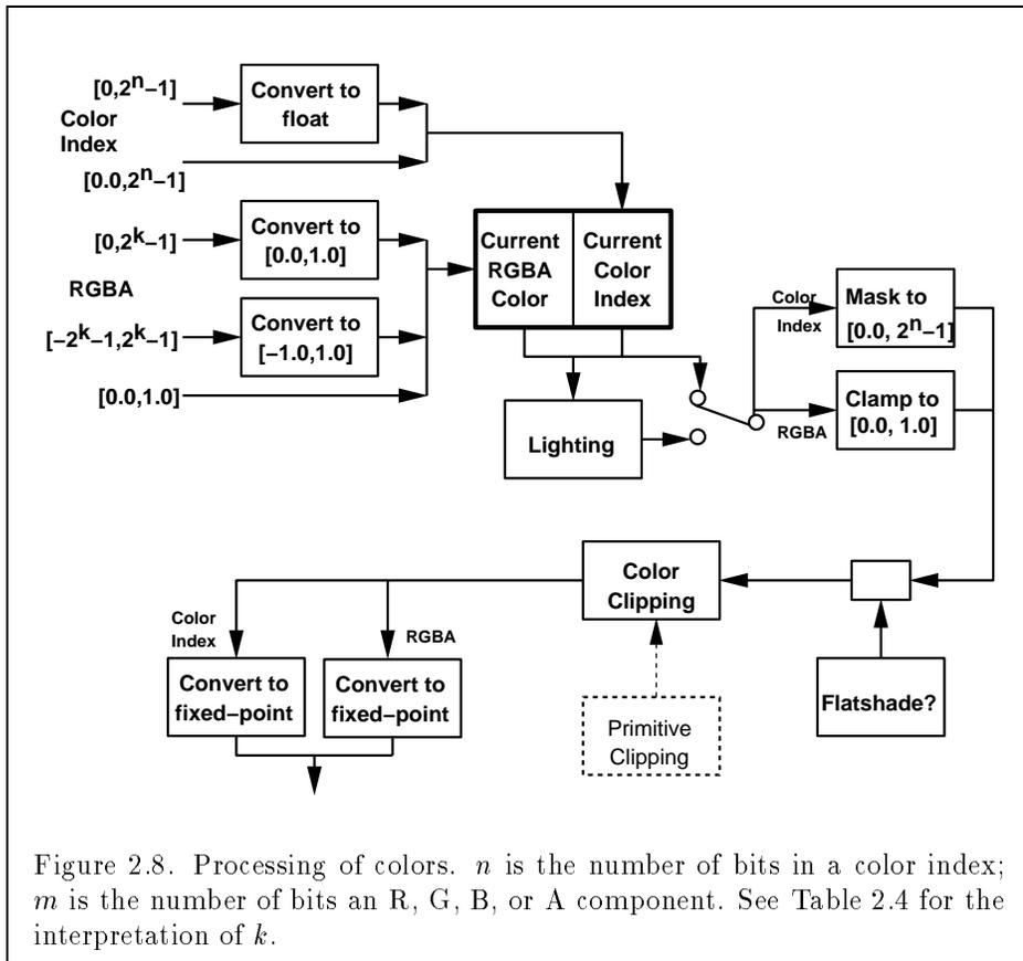
Figure 2.8. Processing of colors.  $n$  is the number of bits in a color index;  $m$  is the number of bits an R, G, B, or A component. See Table 2.4 for the interpretation of  $k$ .
