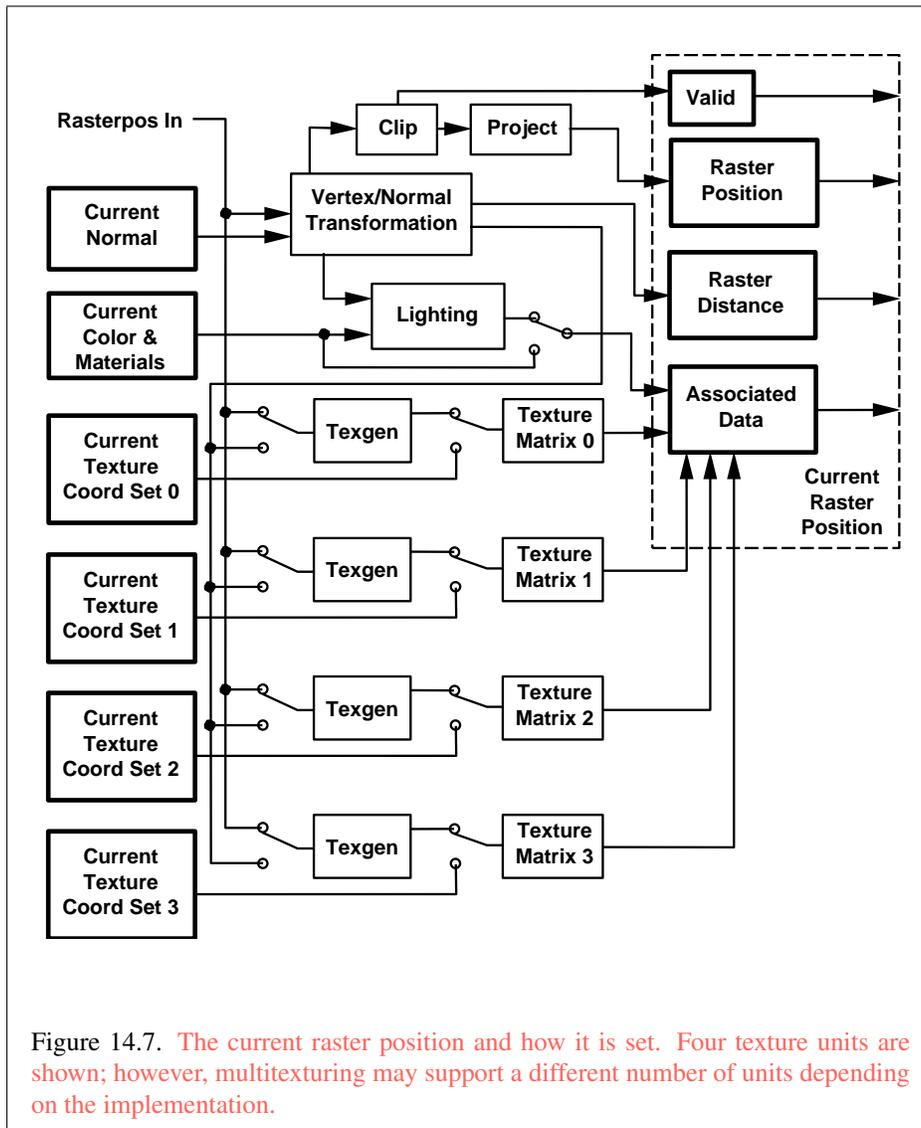
Figure 14.7. The current raster position and how it is set. Four texture units are shown; however, multitexturing may support a different number of units depending on the implementation.
