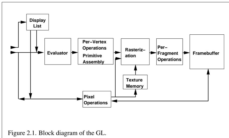
Figure 2.1. Block diagram of the GL.
