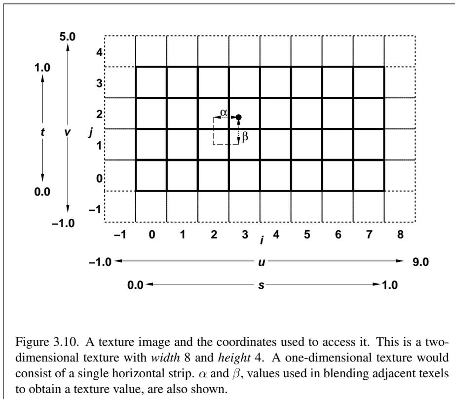
Figure 3.10. A texture image and the coordinates used to access it. This is a two-dimensional texture with *width* 8 and *height* 4. A one-dimensional texture would consist of a single horizontal strip.  $\alpha$  and  $\beta$ , values used in blending adjacent texels to obtain a texture value, are also shown.
