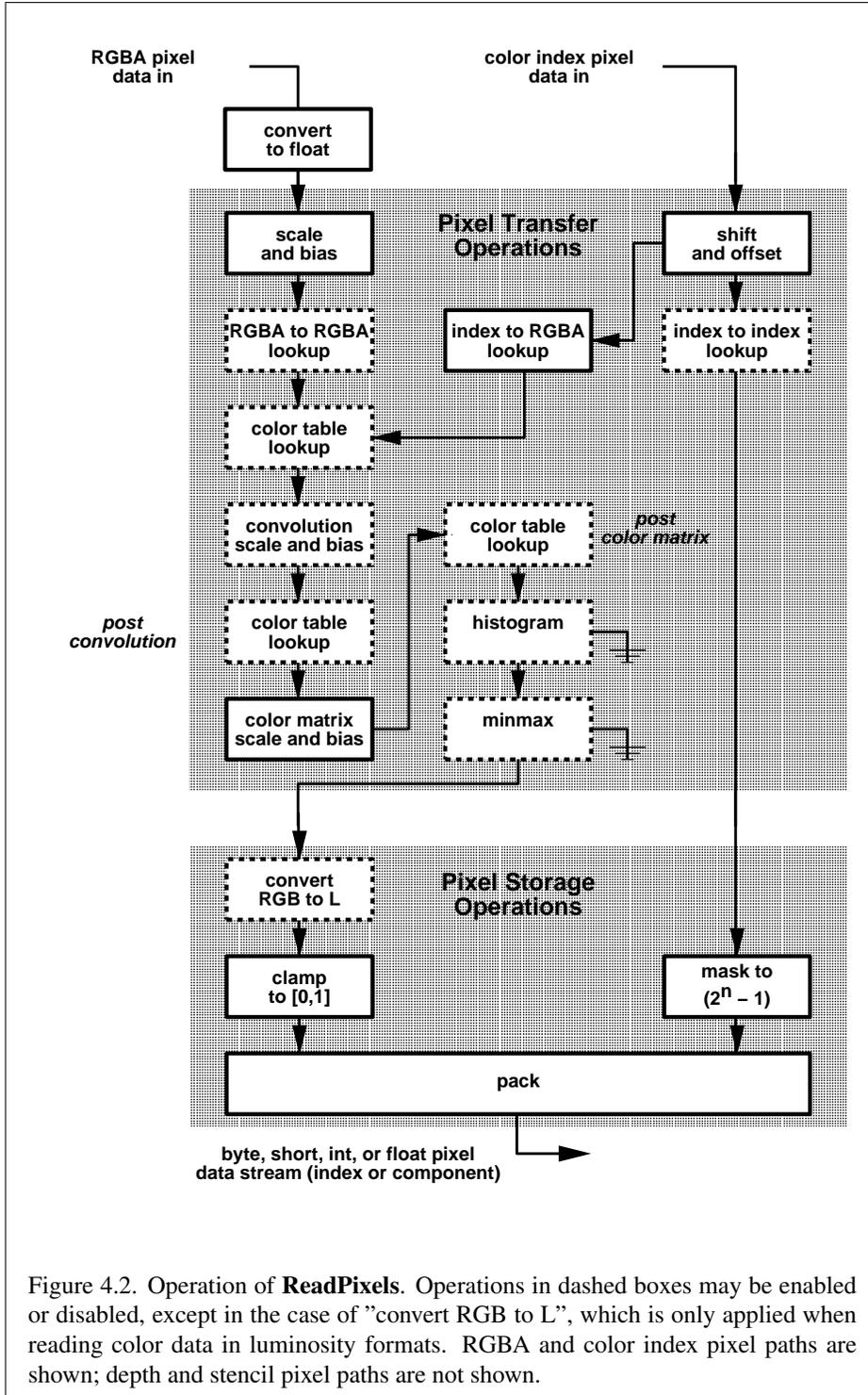
Figure 4.2. Operation of **ReadPixels**. Operations in dashed boxes may be enabled or disabled, except in the case of "convert RGB to L", which is only applied when reading color data in luminosity formats. RGBA and color index pixel paths are shown; depth and stencil pixel paths are not shown.
