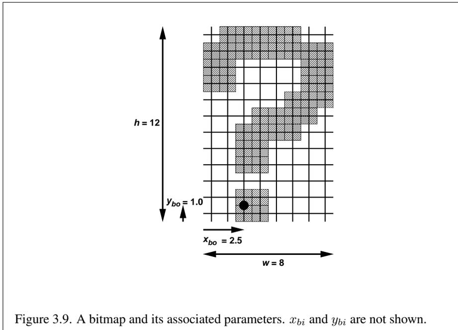
Figure 3.9. A bitmap and its associated parameters.  $x_{bi}$  and  $y_{bi}$  are not shown.
