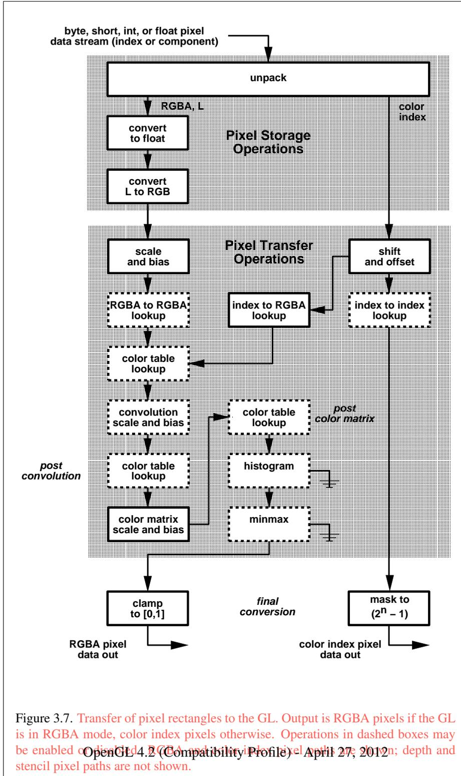
Figure 3.7. Transfer of pixel rectangles to the GL. Output is RGBA pixels if the GL is in RGBA mode, color index pixels otherwise. Operations in dashed boxes may be enabled or disabled. © Khronos Group Inc. All rights reserved. Open GL 4.2 (Compatibility Profile) - April 27, 2012; depth and stencil pixel paths are not shown.
