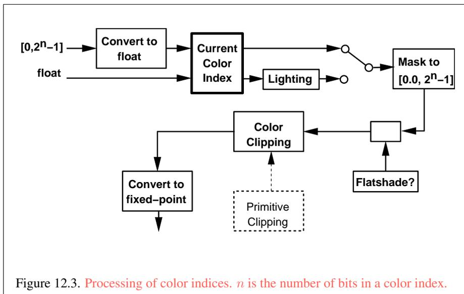
Figure 12.3. Processing of color indices.  $n$  is the number of bits in a color index.
