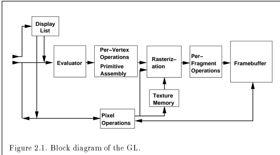
Figure 2.1. Block diagram of the GL.
