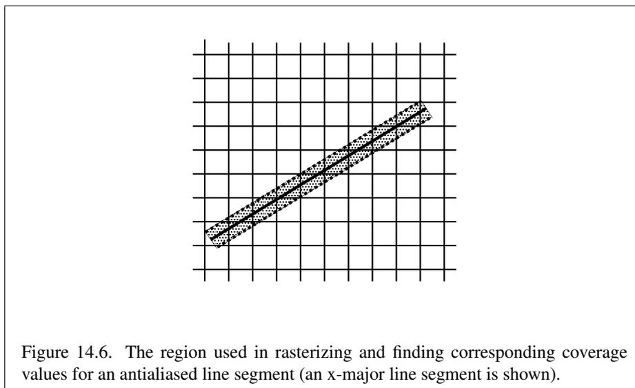
Figure 14.6. The region used in rasterizing and finding corresponding coverage values for an antialiased line segment (an x-major line segment is shown).
