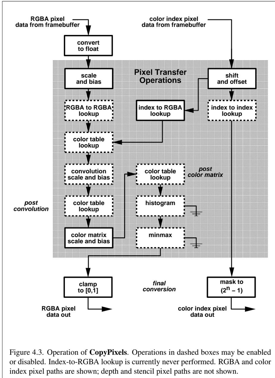
Figure 4.3. Operation of **CopyPixels**. Operations in dashed boxes may be enabled or disabled. Index-to-RGBA lookup is currently never performed. RGBA and color index pixel paths are shown; depth and stencil pixel paths are not shown.
