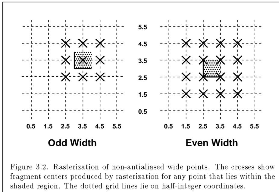
Figure 3.2. Rasterization of non-antialiased wide points. The crosses show fragment centers produced by rasterization for any point that lies within the shaded region. The dotted grid lines lie on half-integer coordinates.
